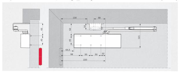
With this fixing method, the max closing force is approx. 20 Nm (for doors up to 950mm)
